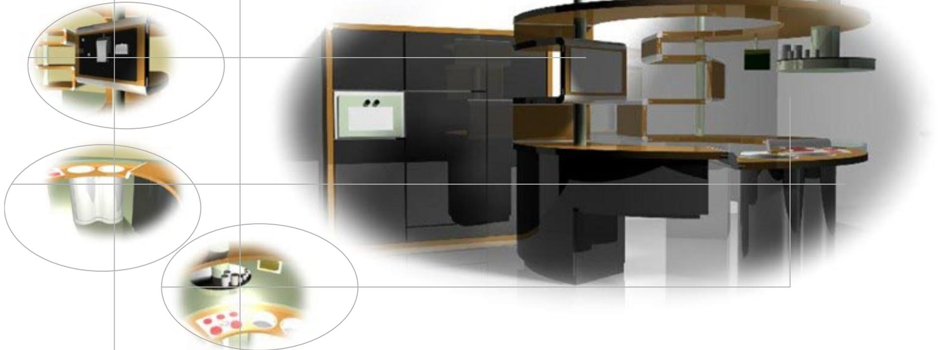
This is the picture of the first CAS visualization of the whole kitchen after several refinements and changes. It should be noticed that the oven, the fridge and the dishwasher had been removed from the kitchen and put in an equipped wall kept apart from the kitchen framework.
